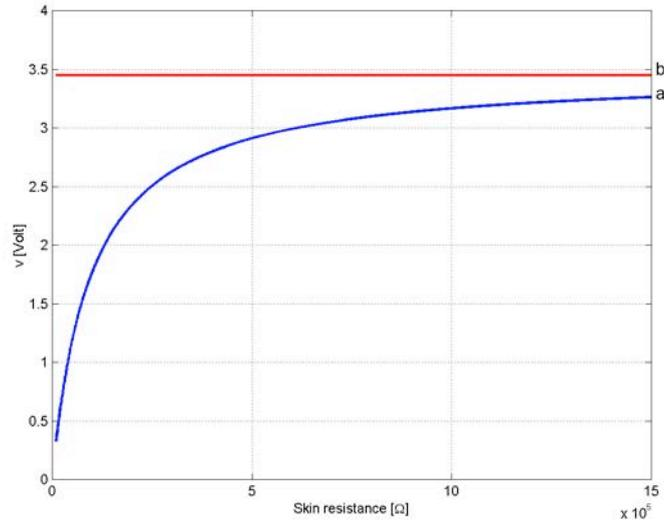
Picture 2. Tension curve  $v$  with respect to skin resistance  $R$  (blue) and the non-contact minimum detectable tension (red).
